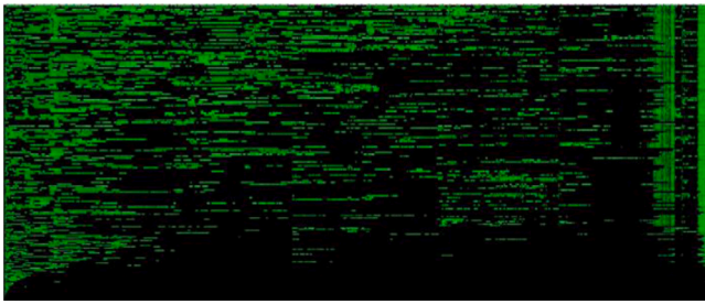
Fig. 3. Load Imbalance in Unbalanced Tree Search using GNU OpenMP and 192 threads (green shows useful work and black shows idle time).
