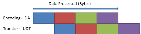
Fig. 7. Pipelining of Encoding and Transferring for a write operation in IStore
